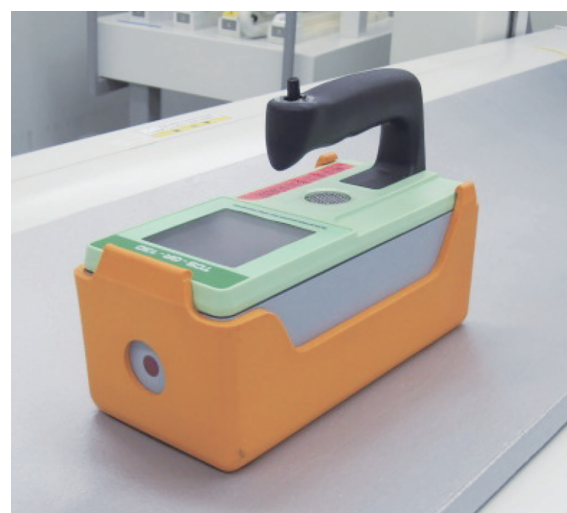
Figure 2 The air dose rate measurement device. Scintillation type survey meter TCS-GD-130.
